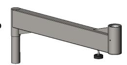
FRAME TUBE: 2" X 4" X .120" WALL [50.8mm X 101.6mm X 3mm] S.S TUBE
